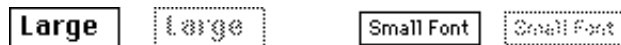
Examples of enabled and disabled fields using large and small fonts on a black and white monitor
