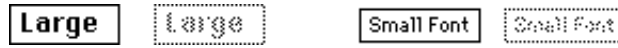
Examples of enabled and disabled fields using large and small fonts on a black and white monitor
