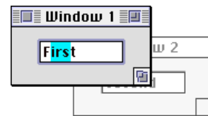
User activates window 1 by clicking on it. Keyboard focus returns to window 1 exactly as it was left.
